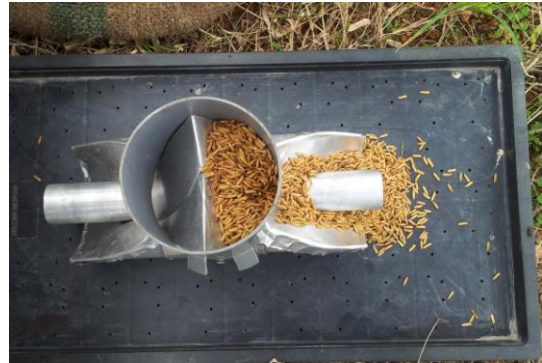
Fig. 4: Grain flow tester
