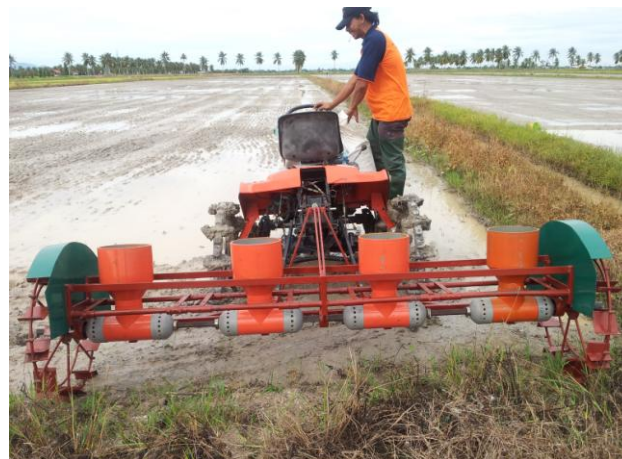
Fig. 1: Seeder machine attach with prime mover
