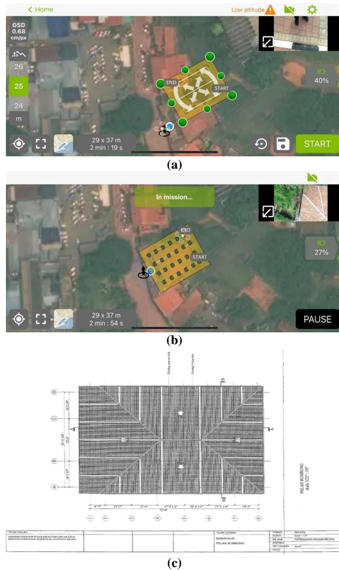
Fig. 1 (a) Area taken from the roof (b) Drone's route on the roof (c) Roof plan
