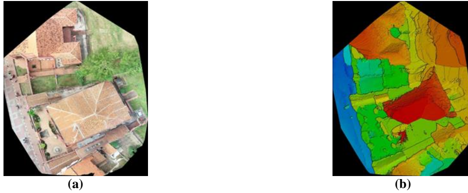
Fig. 2 (a) Orthomosaic and (b) the corresponding sparse Digital Surface Model (DSM) before the densification
