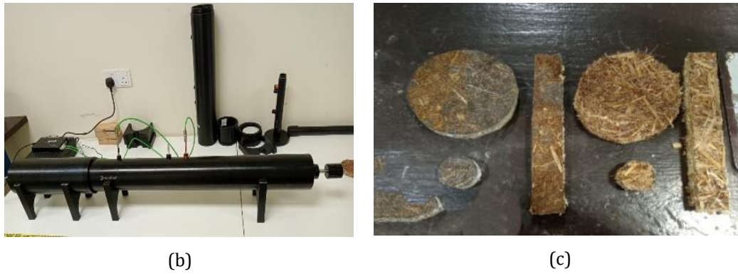
Fig. 4 (a) The process of water absorption test, acoustical test (b) Impedance tube equipment (c) 28mm and 100mm diameter sample
