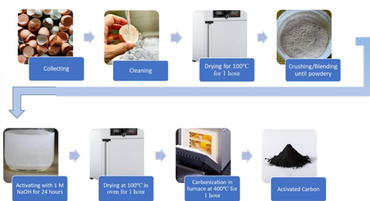
Fig. 1 Production of activated carbon from eggshell
