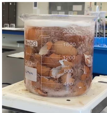
Fig. 1 Eggshells boiled using hotplate stirrer
