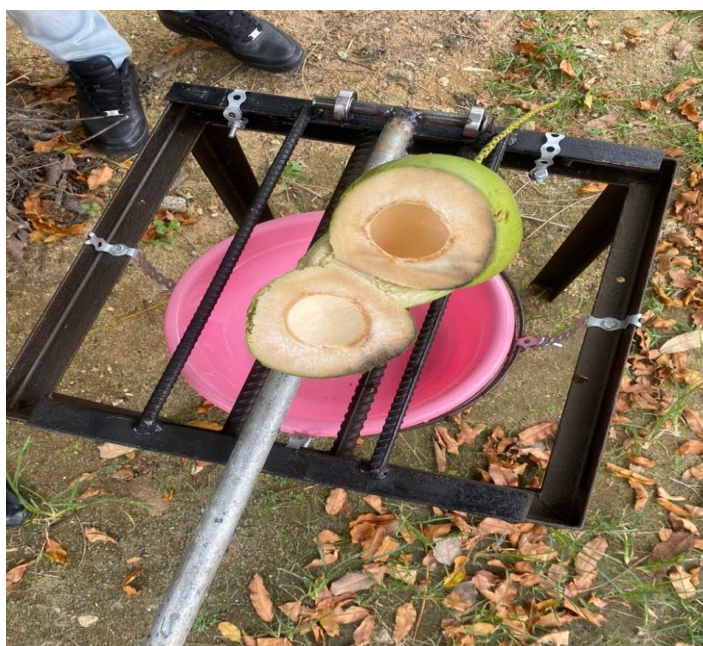
Fig. 4 Cutting time test using Instant Coconut Cutter
