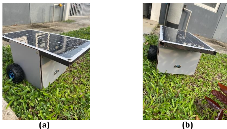
Fig. 5 Final product of Smart Solar Grass Cutter (a) Side view (b) Front view
