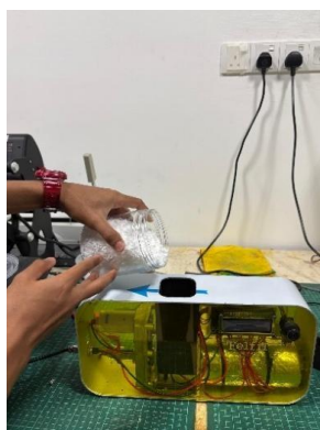
Fig. 3 Filament extrusion using Felfil Evo Pro machine
