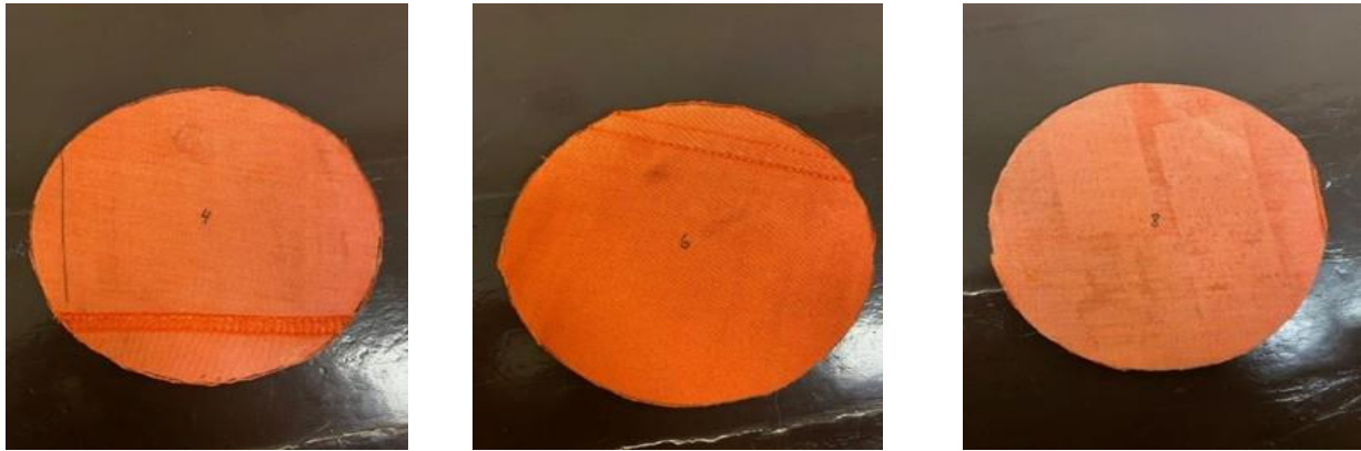
(a) (b) (c) Fig. 2 Sample layers used fabric for the test (i) 4 layers, (ii) 6 layers, (iii) 8 layers
