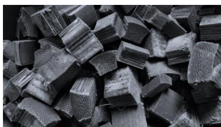
Figure 2: Bamboo Pieces (as Aggregate)
