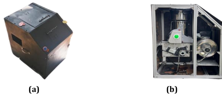
Fig. 2 Mini food waste composter prototype (a) Outer body (b) Internal structure
