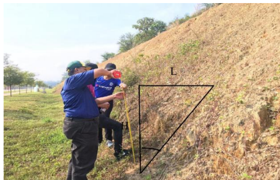
Figure 1 : Manually dimensioning of slope
