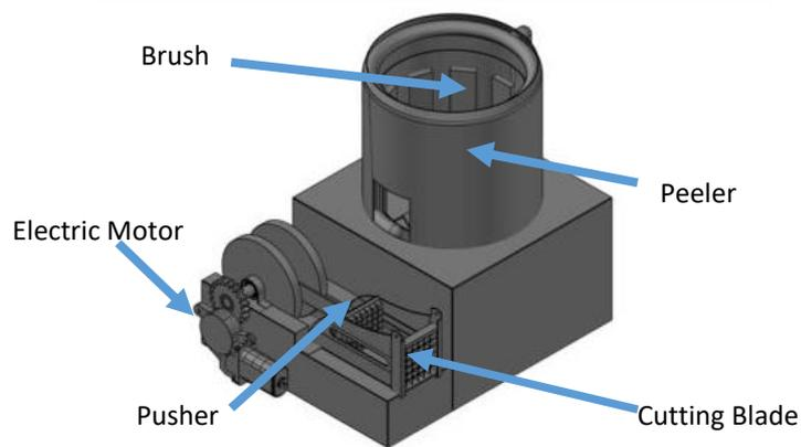
**Figure 2 : Isometric view of Semi-Automatic Potato Peeler and Cutter**
