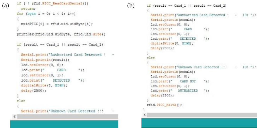
Figure 8: Coding for (a) card detected and (b) not detected
