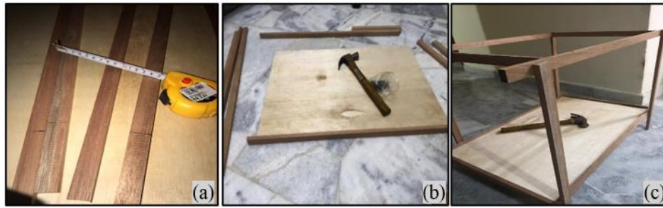
Figure 6: The process of nailing and hammering for the Housing part
