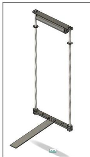
**Figure 5: Pressure Roller Mechanism**
