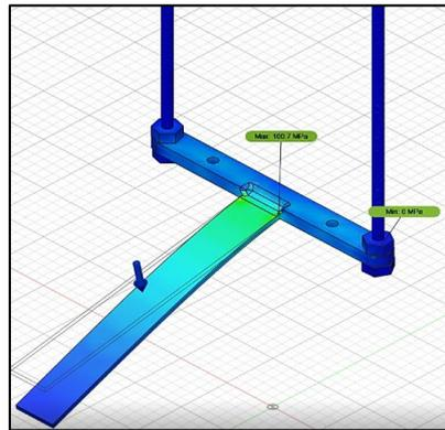
**Figure 11: Stress Test**
