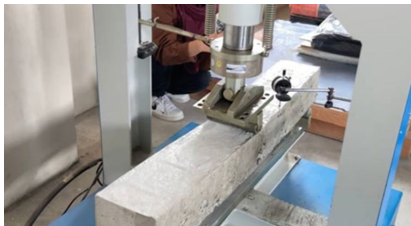
Figure 1: The beam is to be tested using Flexural Compression Test Machines
