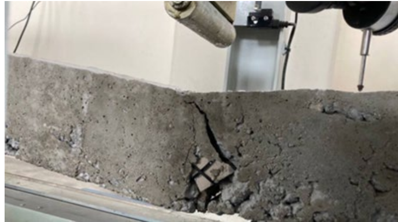
Figure 2: The beam test results were failed using Flexural Compression Test Machines
