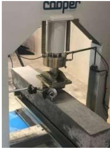
Figure 3: Flexural Strength Test of Beam
