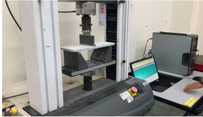
Figure 1: Bending test procedure
