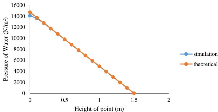
**Figure 6: The comparison of pressure distribution with depth by using hydrostatic pressure between simulation and theoretical value**
