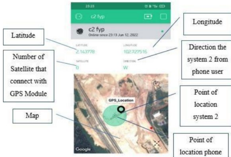
Figure 9: Location of fire extinguisher is displayed in Blynk app
