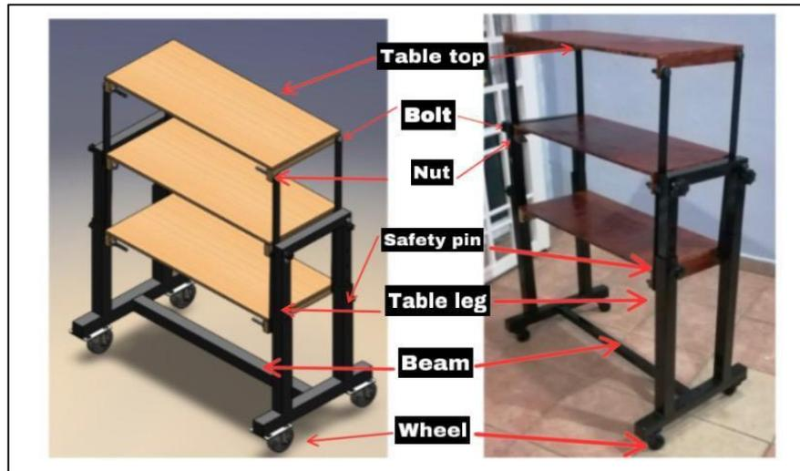
**Figure 4: Design of the part for the Convertible Table and Shelf**
