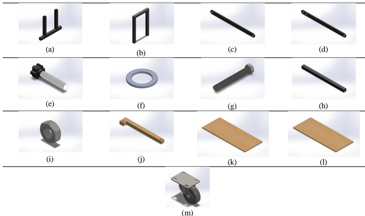
**Figure 1: Design parts (a) Base, (b) Adjustable base, (c) Handle 1, (d) Handle 2 (e) Safety pin, (f)Washer, (g) Bolt, (h) Connector, (i) Nut, (j) Side panel, (k) Top panel 1, (l) Top panel 2, (m) Wheel**
