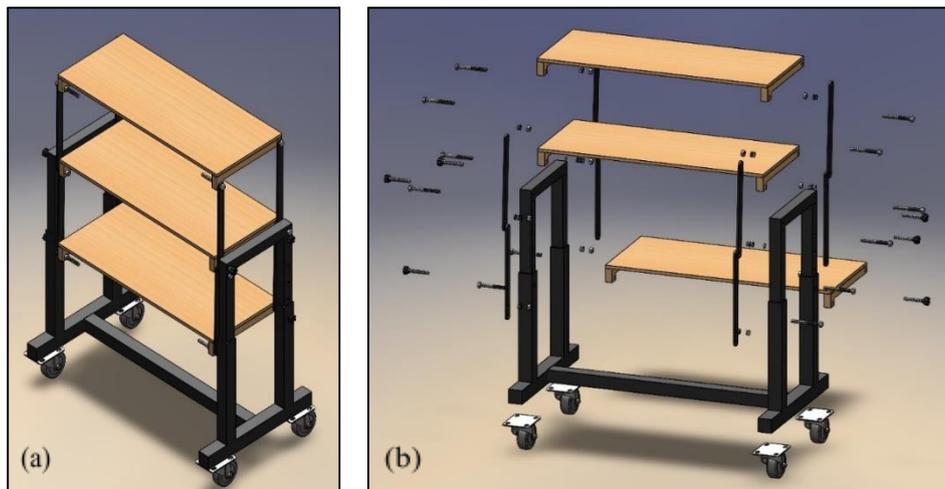
**Figure 2:** (a) Assembly design and (b) Exploded view
