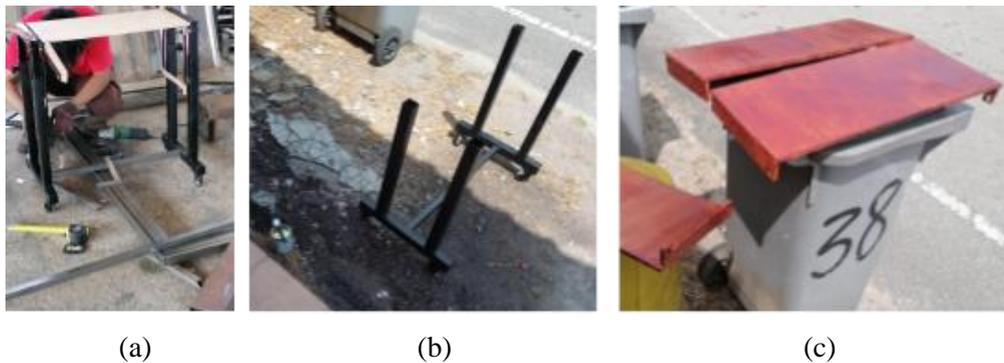
**Figure 3: Fabrication process of convertible table and shelf, (a) The hollow section getting welded together, (b) The hollow section painted black, (c) The panel with wood varnish**
