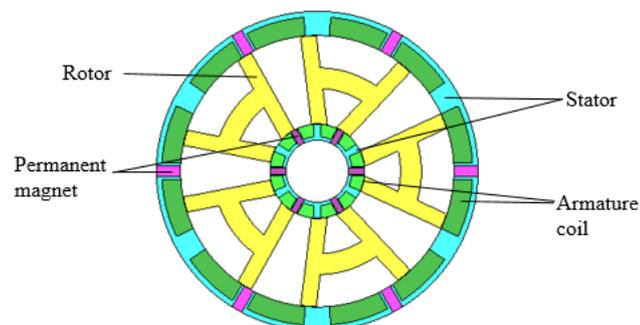
**Figure 1: The proposed design of H-configuration modular rotor PMFSM**
