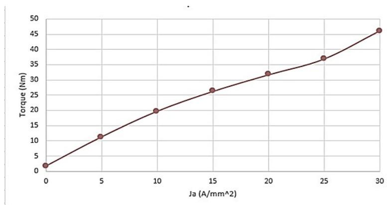
**Figure 5: Torque versus current density**
