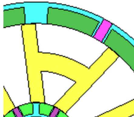
**Figure 3: H-configuration modular rotor PMFSM**
