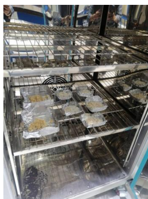
Figure 3: Rice samples were oven dried at 65°C for 72 hours
