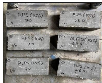
Figure 6: The sample of sand cement bricks with paper sludge
