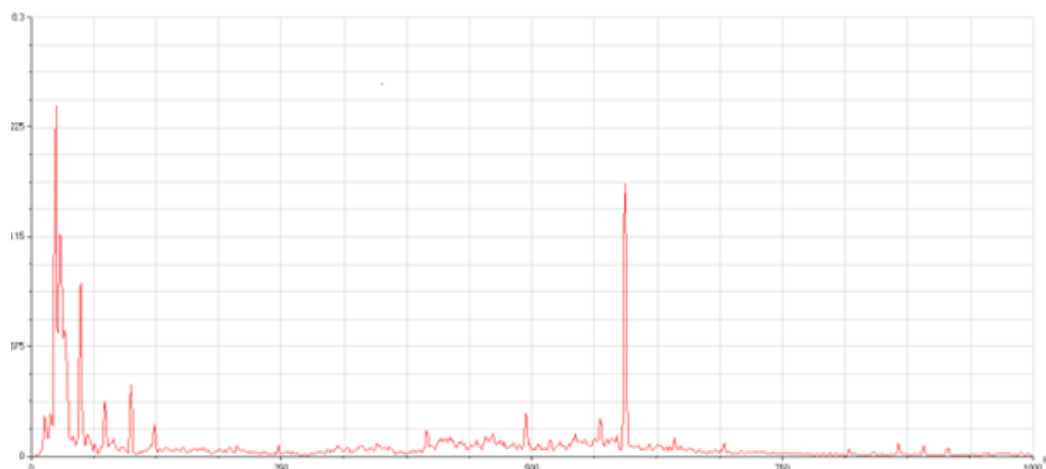
Figure 7 Horizontal vibration spectrum for pump D at Point 2
