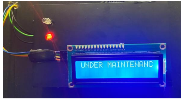
Figure 8: The LCD1 display “UNDER MAINTENANC”
