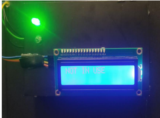
Figure 3: The LCD1 display “NOT IN USE”
