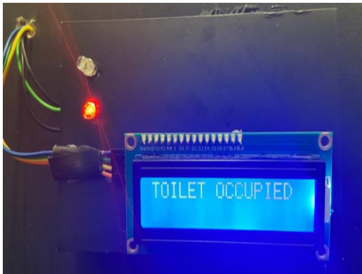
Figure 4: The LCD1 display “TOILET OCCUPIED”
