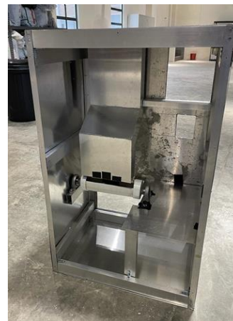
Figure 2: Beverage storage and dropping mechanism
