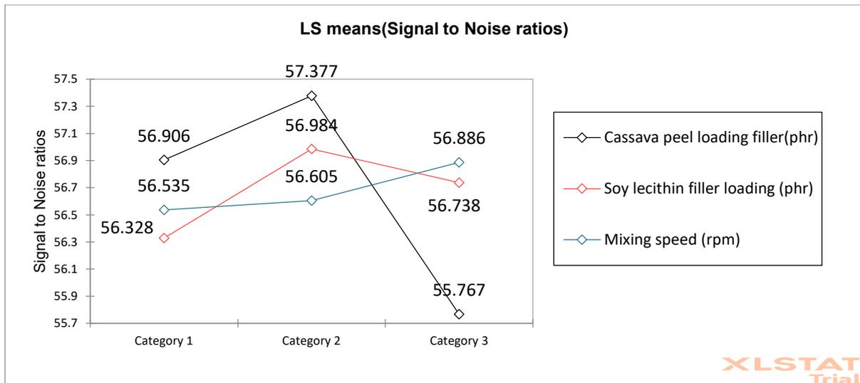
**Figure 3.2:** Signal Noise (SN) plot of stress at break for prepared films
