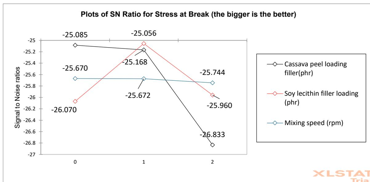
**Figure 3.2:** Signal Noise (SN) plot of stress at break for prepared films
