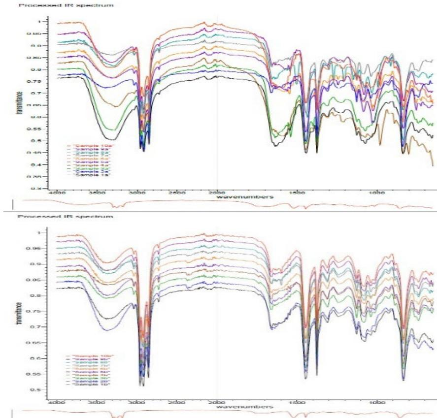
**Figure 3.1:** FTIR spectra of the cassava-peel starch loaded NRL films before soil burial test and after soil burial test.
