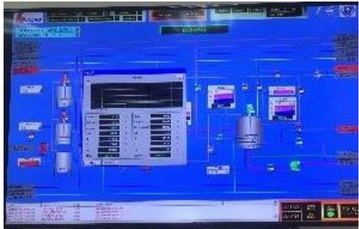
Figure 2: SCADA system used at Biodiesel Pilot Plant in the control system
