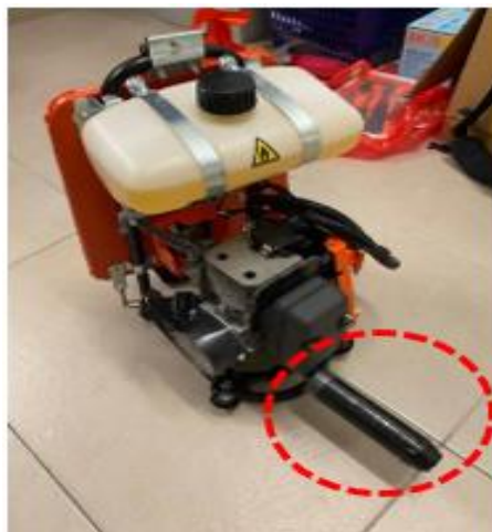
Figure 7: Positioning of silencer on grass trimmer
