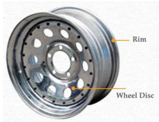
Figure 1: Part of wheel and rim [5]
