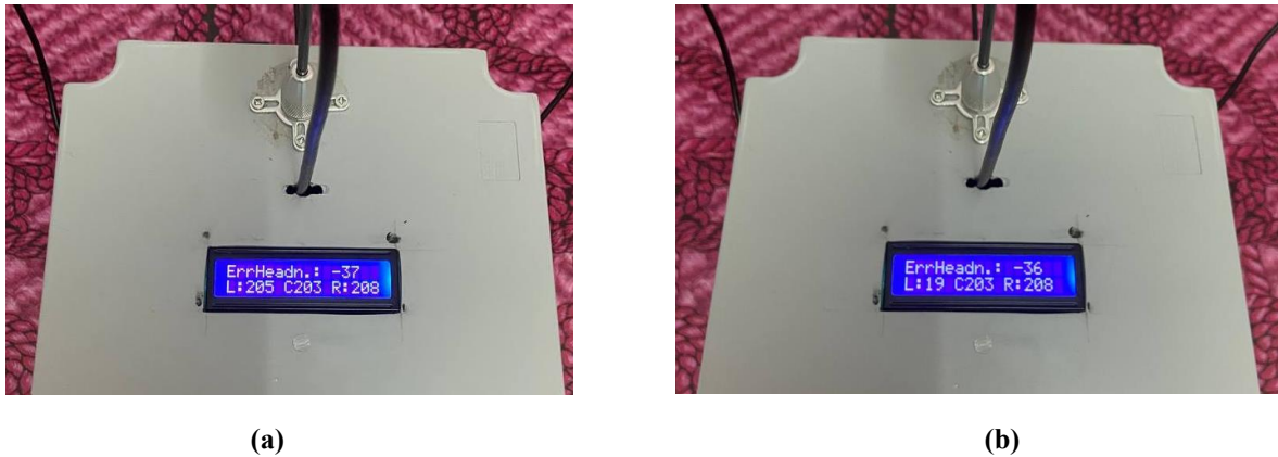
Figure 7: (a) No obstacle detected; (b) Left sensor detect an obstacle
