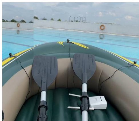
Figure 6: The position of left, right and middle waterproof ultrasonic sensor
