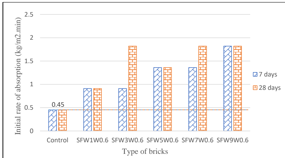
Figure 7: Initial rate of absorption of cement bricks for 7 days and 28 days
