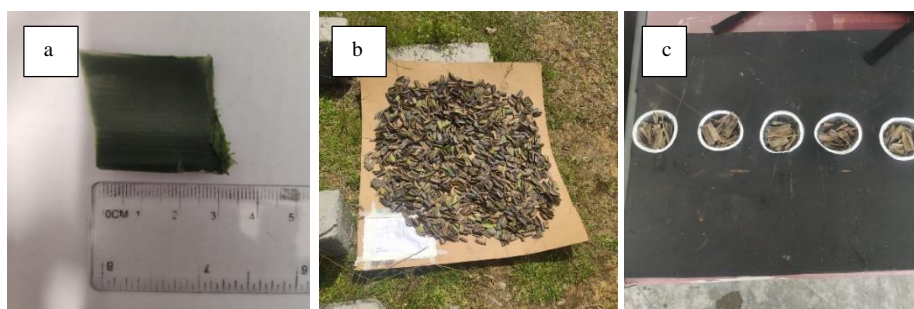
Figure 1: (a) 3 cm long pineapple leaf (b) drying process (c) moisture content analysis sample
