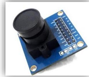
**Figure 15: OVA7670 Camera module without FIFO-VGA-30fps**
