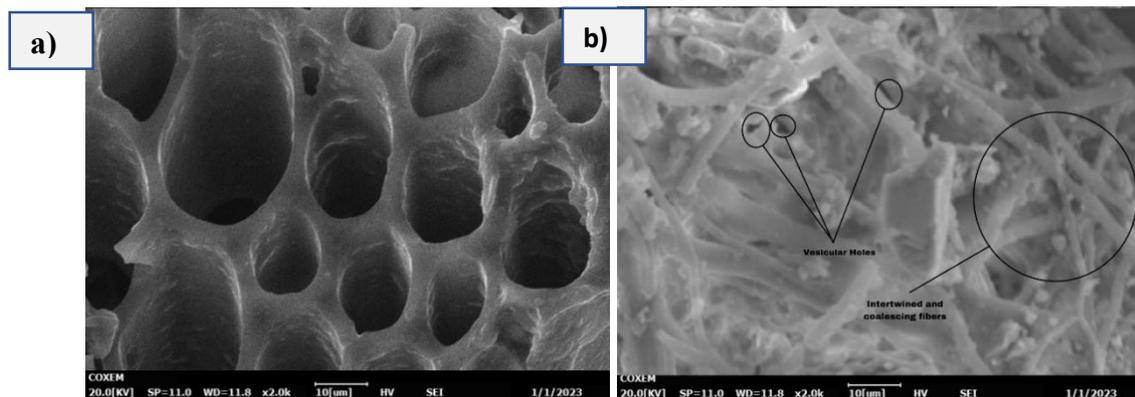
Figure 4.5 SEM Imaging of Sugarcane Bagasse with x2.0k Magnification Fixed
