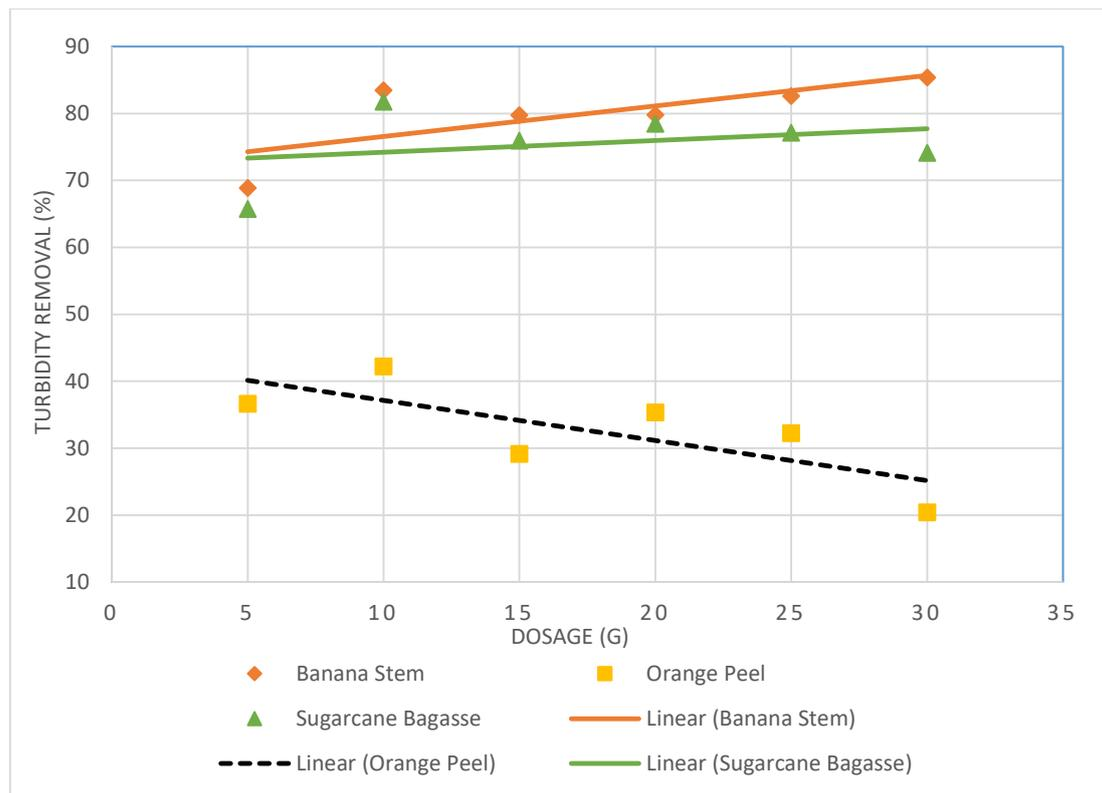
Figure 4.11: Effect of Adsorbent Dosage on Turbidity Removal.
