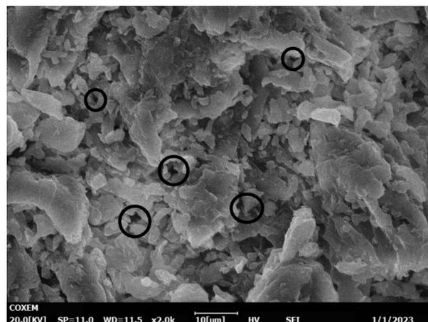
Figure 4.6 SEM Imaging of Orange Peel with x2.0k Magnification Fixed
