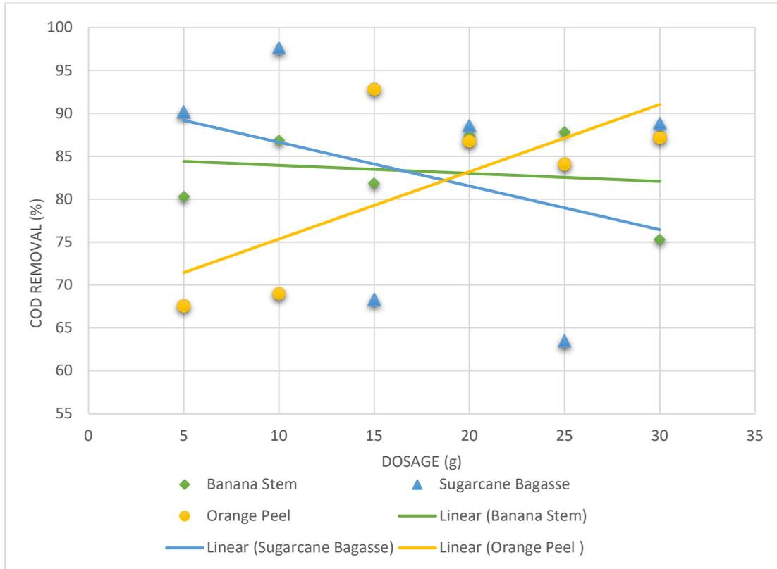
Figure 4.13: Effect of Adsorbent Dosage on COD Removal.
