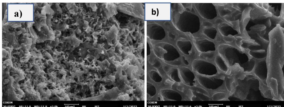
Figure 4.4: SEM Imaging of Banana Stem with x2.0k Magnification Fixed
