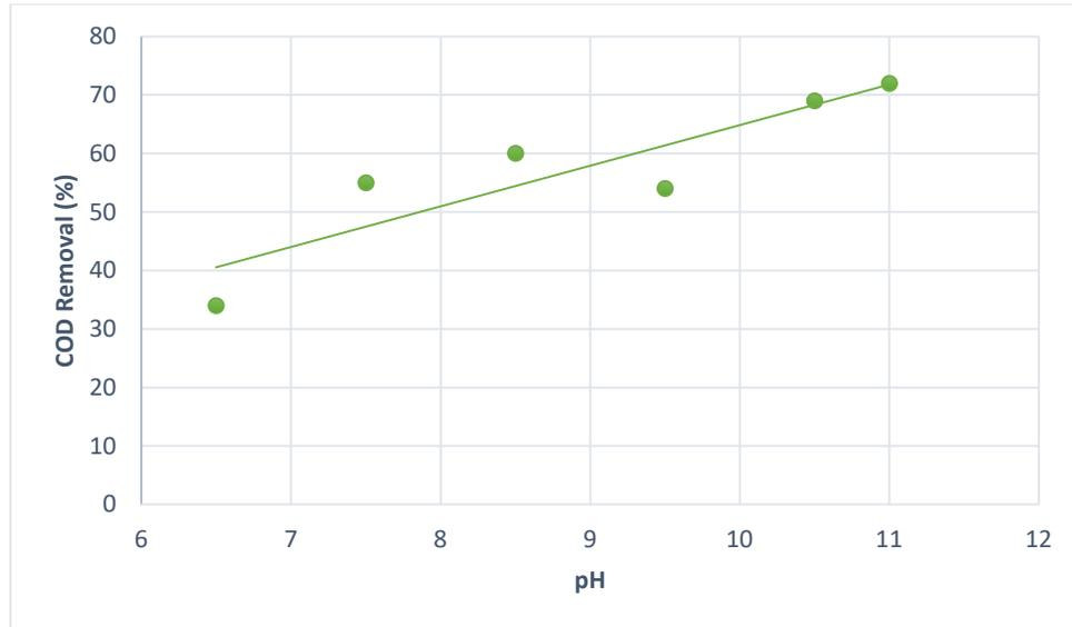
Figure 4.10: Effect of pH on COD Removal.
