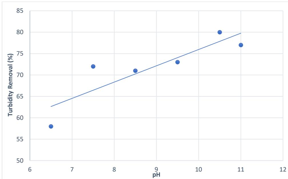
Figure 4.8: Effect of pH on Turbidity Removal.
