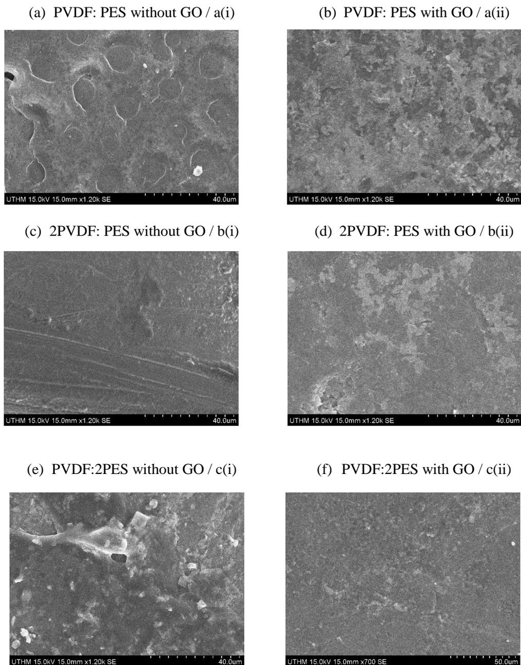
**Figure 3.4 SEM images of top surface UF membranes (a) PVDF: PES without GO / a(i), (b) PVDF: PES with GO / a(ii), (c) 2PVDF: PES without GO / b(i), (d) 2PVDF: PES with GO / b(ii), (e) PVDF:2PES without GO / c(i), (f) PVDF:2PES with GO / c(ii)**
