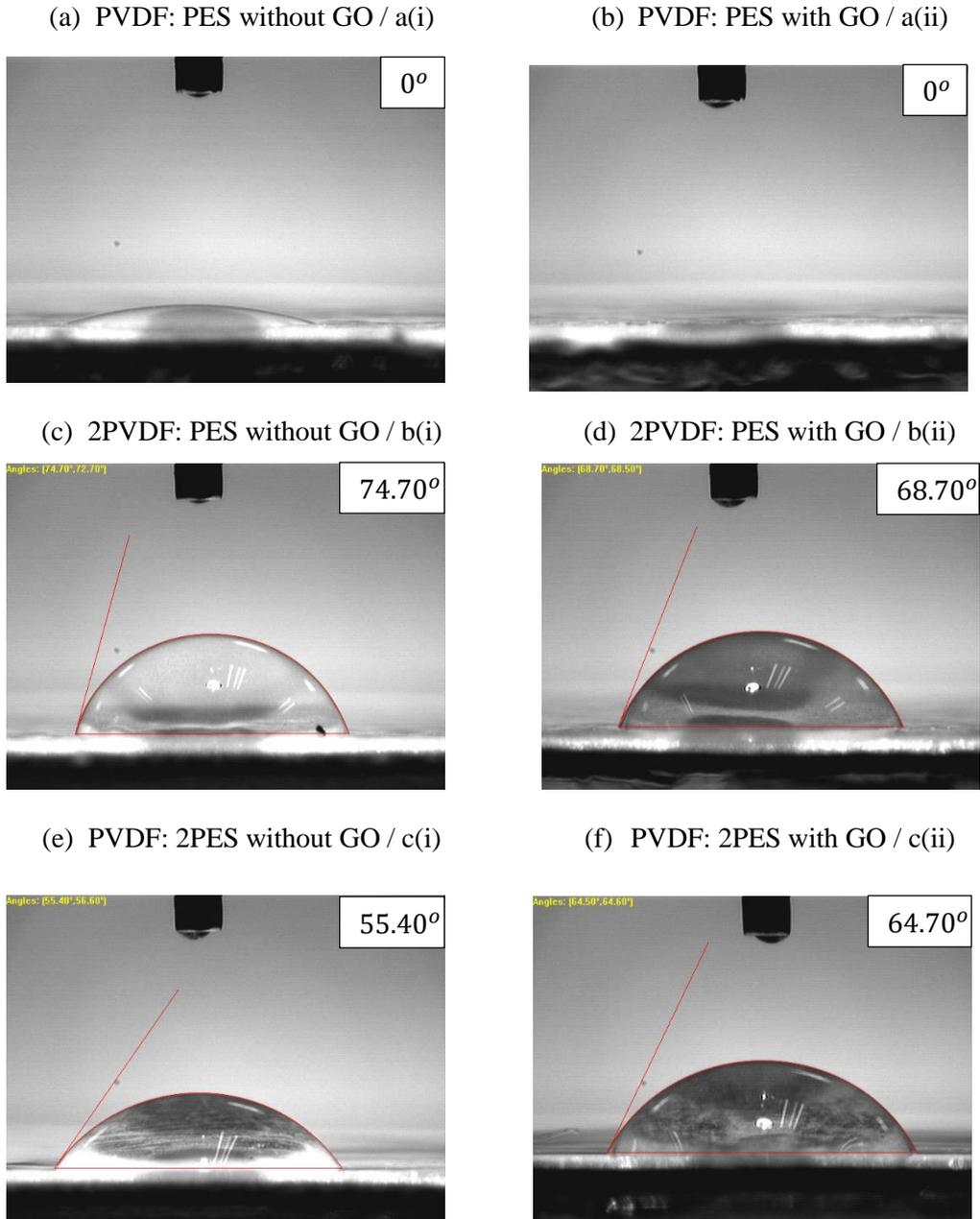
**Figure 3.5: Contact angle water droplet on UF membrane (a) PVDF: PES without GO / a(i), (b) PVDF: PES with GO / a(ii), (c) 2PVDF: PES without GO / b(i), (d) 2PVDF: PES with GO / b(ii), (e) PVDF:2PES without GO / c(i), (f) PVDF:2PES with GO / c(ii)**
