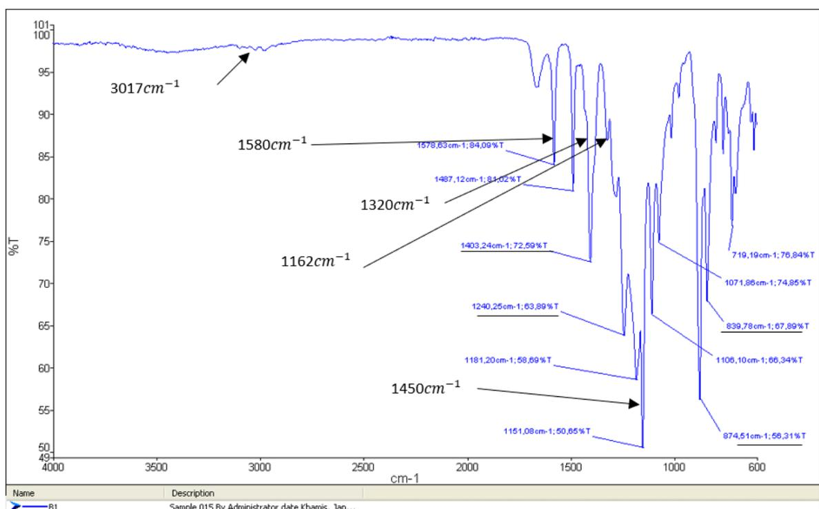
Figure 3.2: IR spectrum for 2PVDF: PES without GO / b (i)
