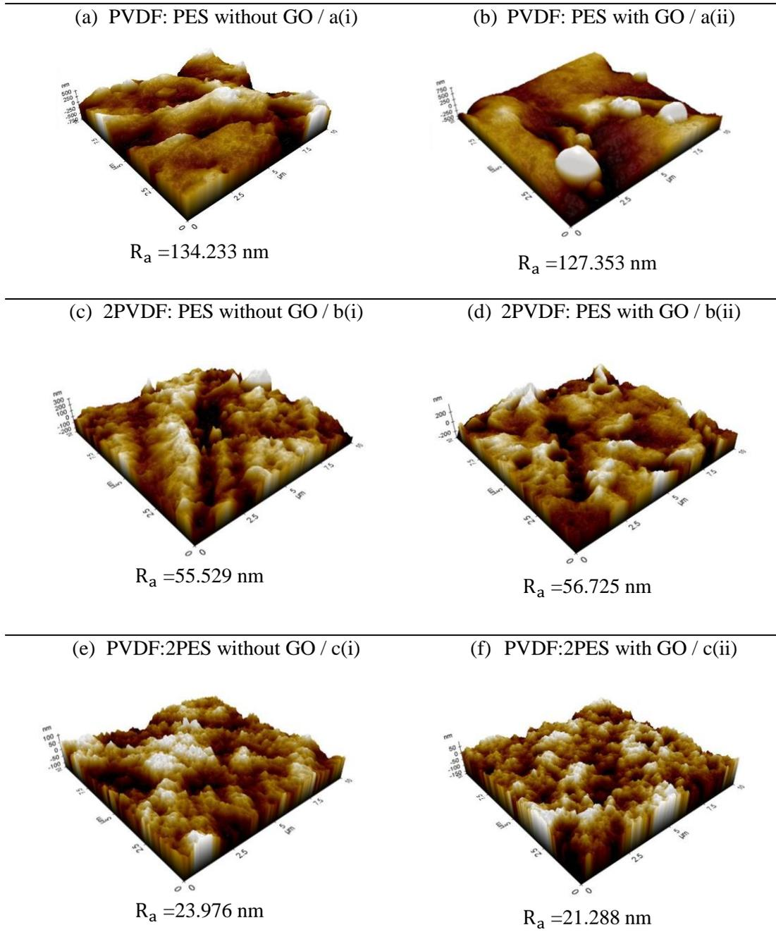
**Figure 3.1: AFM topographic images of UF membranes (a) PVDF: PES without GO / a(i), (b) PVDF: PES with GO / a(ii), (c) 2PVDF: PES without GO / b(i), (d) 2PVDF: PES with GO / b(ii), (e) PVDF:2PES without GO / c(i), (f) PVDF:2PES with GO / c(ii)**
