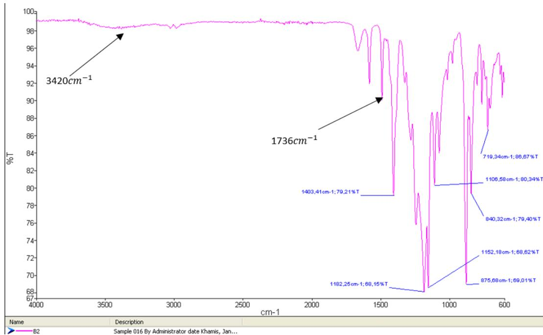
**Figure 3.3: IR spectrum for 2PVDF: PES with GO / b (ii)**
