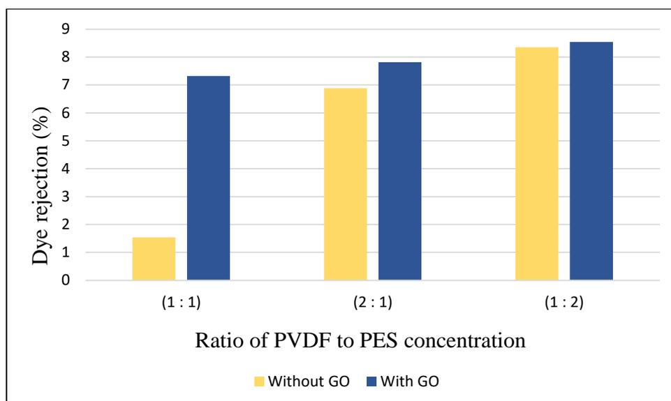
**Figure 3.8: Dye rejection (%) against ratio of PVDF to PES concentration without and with GO**
