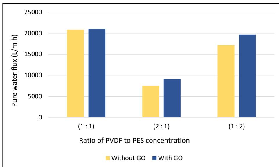
**Figure 3.6: Pure water flux (L/m<sup>2</sup>h) against Ratio of PVDF to PES concentration without and with GO**
