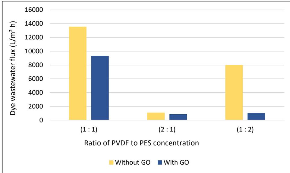
**Figure 3.7: Dye wastewater flux (L/m<sup>2</sup>h) against Ratio of PVDF to PES concentration without and with GO**
