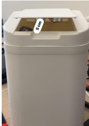
Figure 7: Trash at 5 cm from Ultrasonic Sensor
