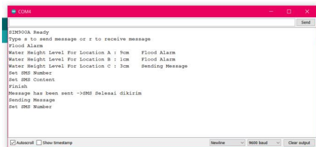
Figure 10 : Result of three ultrasonic systems on Serial Monitor
