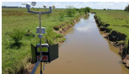
Figure 1: Early flood detection and warning system in Argentina developed with Libelium sensors technology. [14]
