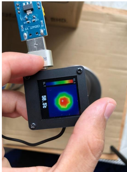
Figure 3.1: Thermal Camera AMG8833 detecting heat
