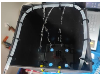
Figure 6: DC Motor Pump Triggered
