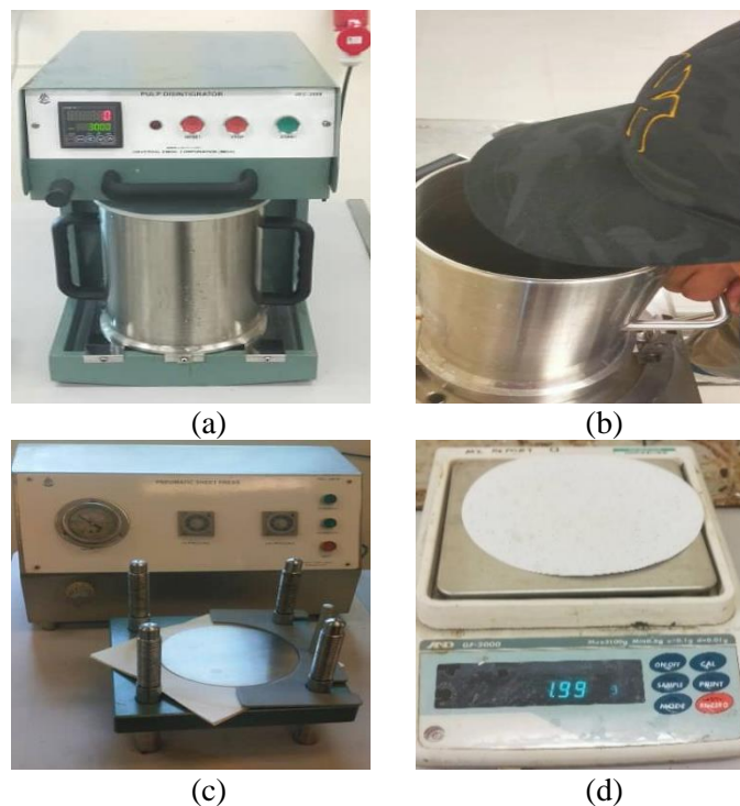
Figure 2: (a) Blending the pulp, (b) Paper formatting process, (c) Pressing Process, (d) Paper weight
