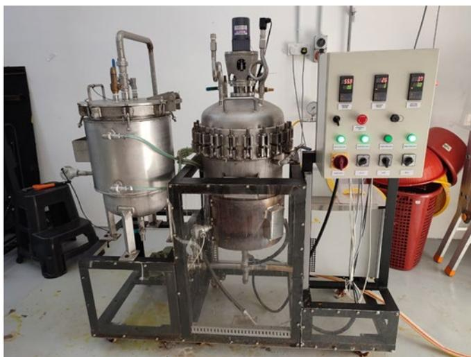
**Figure 1:** The 70 L subcritical water extractor
