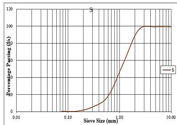
Figure 3: Sieve analysis of sand
