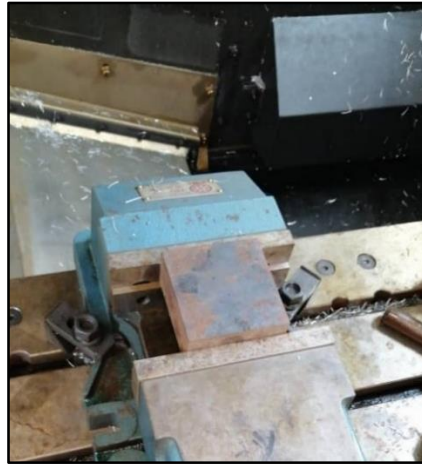
Figure 1: Set up the workpiece on vice
