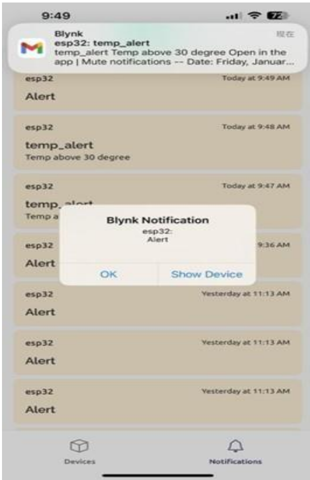
Figure 3: Alert notification given from the blynk application
