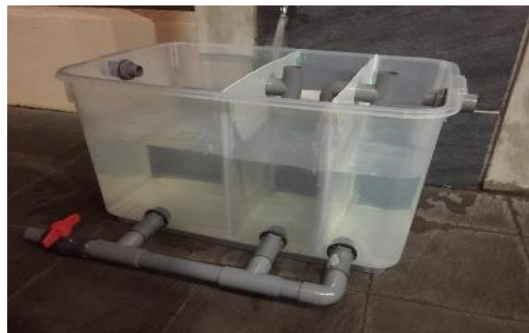
Figure 4: Portable treatment system
