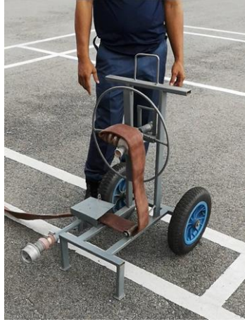
Figure 8: Pagoh Station's Fire hose roller
