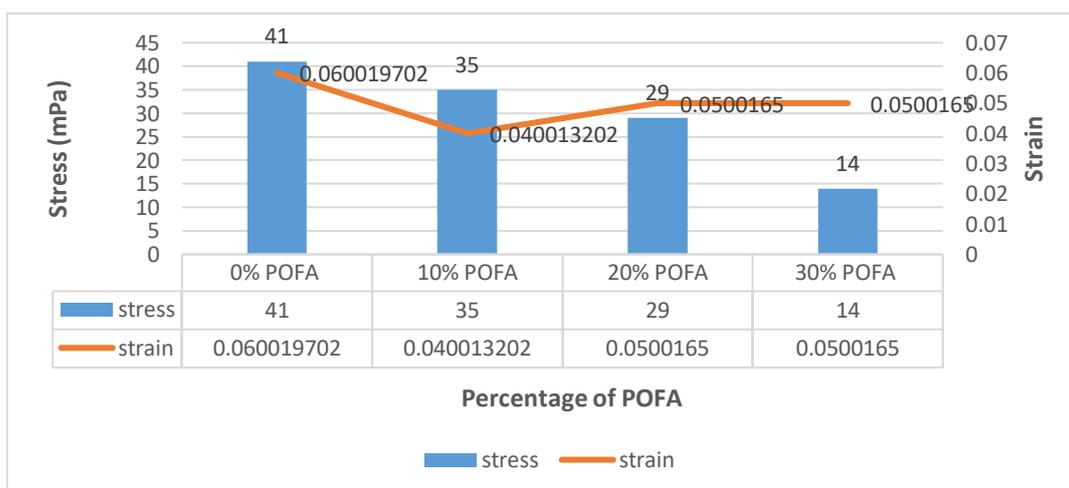
**Figure 4: Highest Value of Stress and Strain on concrete cube containing 0.0 % , 10.0 %, 20.0 % and 30.0 % of POFA**
