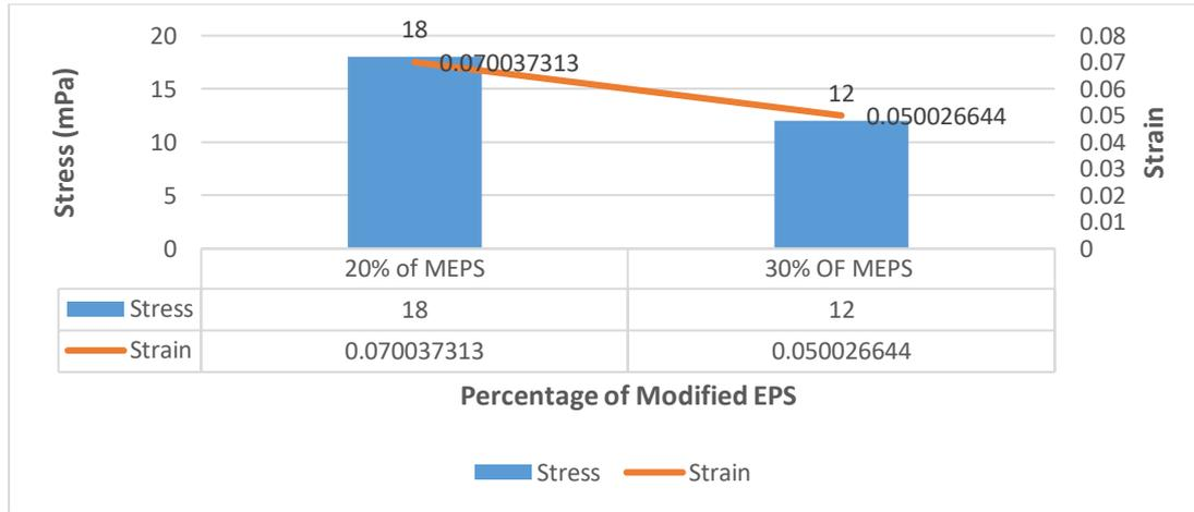
**Figure 5: Highest Value of Stress and Strain on concrete cube containing 20.0 % Modified EPS and 30.0 % Modified EPS**
