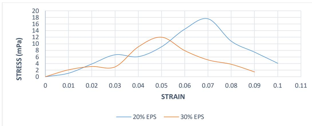
**Figure 3: Relationship of Stress and strain on concrete cube containing 20.0 % Modified EPS and 30.0 % Modified EPS**
